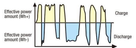
Charge current amount Ah (power amount Wh) and discharge current amount Ah (power amount Wh) can be integrated, respectively.
