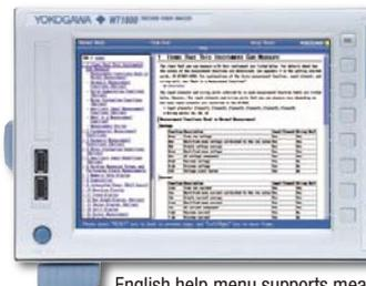
Display the manual on the screen. Frequently used functions (keys) can be performed without the instruction manual. You may, however, want to use a new function during evaluation. The WT1800 includes a built-in instruction manual on the functions, so if a new operation is required, you can read the explanation of the function on the screen.
