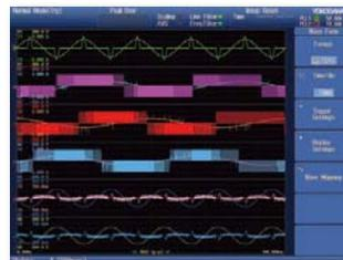
A high resolution display makes it possible to split the waveform display into up to 6 split screens. This makes it possible to split the display of signals between the input and output of a three-phase inverter and display them simultaneously. Waveform display allows you to display waveforms for the voltage alone or the current alone, or arbitrarily set the display position, so you can also display only the signals you want to compare one above the other.
