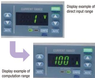
The setting ranges of voltage and current are usually displayed with voltage and current signal levels that are input to the power analyzer. The WT1800 provides not only this direct display but also added a new computation range display function to the external current sensor range. This function allows you to display the primary current range for the voltage output type current sensor. It allows you to intuitively set a range that is suited to the primary measurement signal level.
