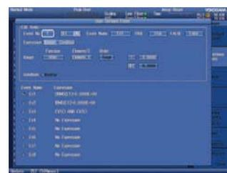
The data saving function of the WT Series is capable of continuously saving data for a long period of time. However, to check an irregular event, data must be retrieved using spreadsheet software. The event trigger function allows you to set the high and low limits and only trigger data that falls into or out of that range to be saved.
