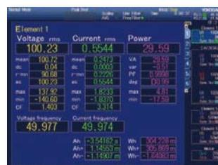
Image data can be loaded onto the screen and the position and size of the numerical data can be specified. The display screen can be customized so that the corporate logo of your company is displayed on the screen, or only the measurement items you want to view, such as input and output efficiency or frequency, are displayed one above the other.
