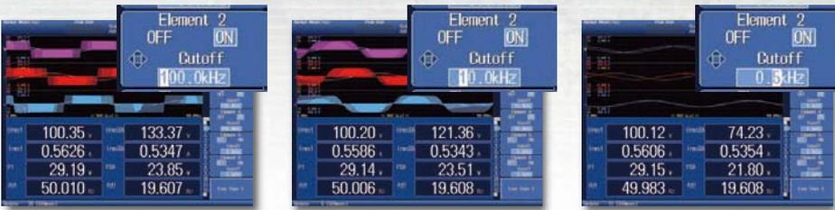
In power evaluation such as an inverter waveform and distorted waveform, measurement values are affected by high frequency component. A new digital filter function makes it possible to remove unnecessary high frequency components superimposed on signals. A filter can be independently set for each input element. An analog filter for 1 MHz/300 kHz, and digital filter that can be set from 100 Hz to 100 kHz in increments of 100 Hz are available as standard.
