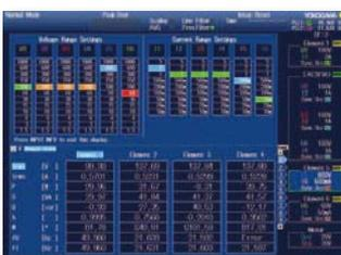
The screen can be split into two, with one above the other, and two types of screens can be displayed simultaneously. Screen can be selected from Numerical, Waveform, Trend, Bar Graph, and Vector displays. Another new function allows you to press the INFO button on the Numerical screen to display the setting information in the upper row and automatically scale down the numerical information displayed in the lower row.
