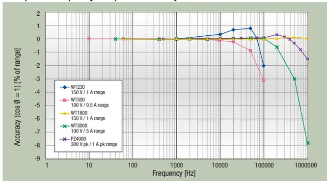
Total power error with rated range input for an arbitrary power factor (at 50/60 Hz)
