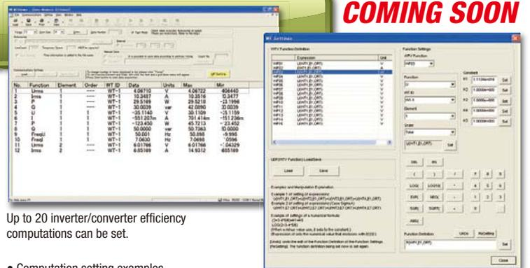
Up to 20 inverter/converter efficiency computations can be set.
