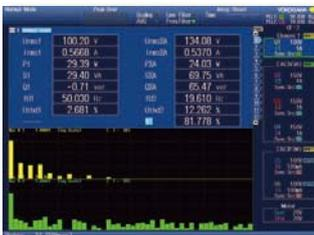
A harmonic measurement option (/G5) makes it possible to display both numerical data and bar graphs to help understand measurement data visually. In addition, a dual harmonic measurement function (/G6) makes it possible to measure and display two-line harmonic bar graphs (dual harmonic) simultaneously.
