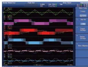
A high resolution display makes it possible to split the waveform display into up to 6 split screens. This makes it possible to split the display of signals between the input and output of a three-phase inverter and display them simultaneously. Waveform display allows you to display waveforms for the voltage alone or the current alone, or arbitrarily set the display position, so you can also display only the signals you want to compare one above the other.
