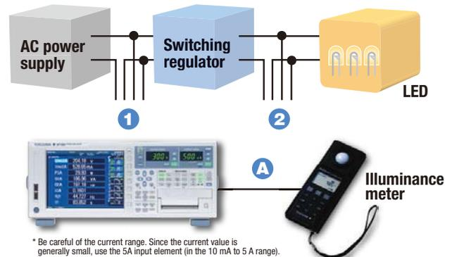
\*Be careful of the current range. Since the current value is generally small, use the 5A input element (in the 10 mA to 5 A range).
