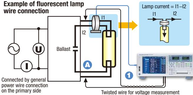
\*Lamp current can be obtained either by measuring the output of a wide range current sensor as shown in the figure, or by obtaining the differential current using computation (delta computation function).
