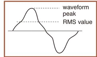
When checking the measurable crest factor of our power measuring instruments, please refer to the following equation.
