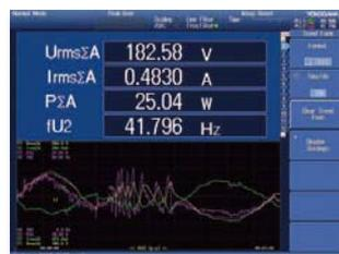
When evaluating inverter efficiency, sometimes small efficiency changes can hardly be recognized with just numerical values. Trend display makes it possible to display measurement values and measurement efficiency as trend data in time series to help capture even small changes visually. Trend data over several minutes or several days can be displayed.
